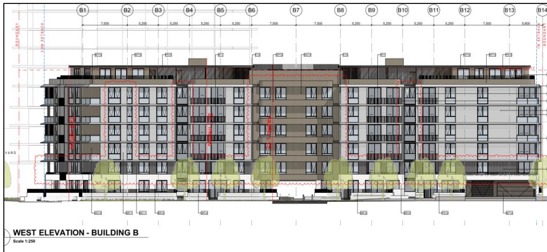
Figure 4: An excerpt from the suite of plans, depicting the building height encroachments above the red-dashed horizontal line.
